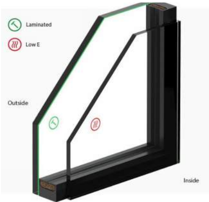
DOUBLE GLAZED LOW-E WINDOW GLAZING SYSTEM
