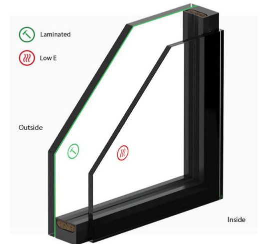
DOUBLE GLAZED LOW-E WINDOW GLAZING SYSTEM
