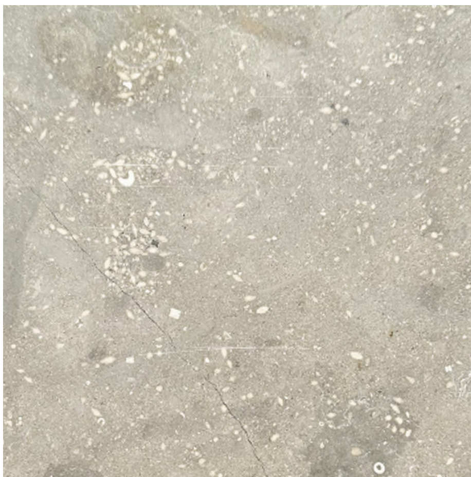
EXTERIOR STONE SLAB CLADDING NAIROBI GRAY LIMESTONE
