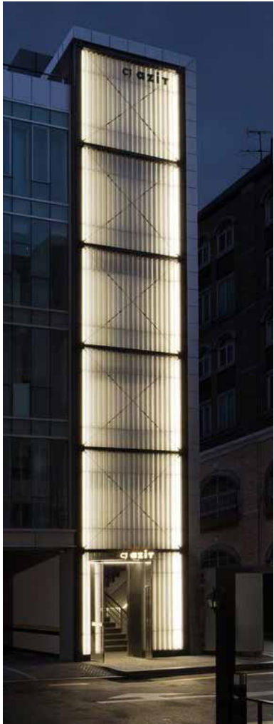
4 FRITTED GLASS OR FLUTED BACKLIT GLASS STAIR TOWERS ALONG MILLWARD ST.
