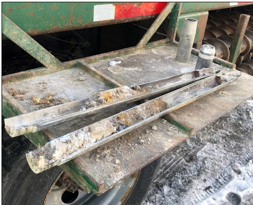
Figure 4: BH-3 Split spoon sample from 21.5' bgs
