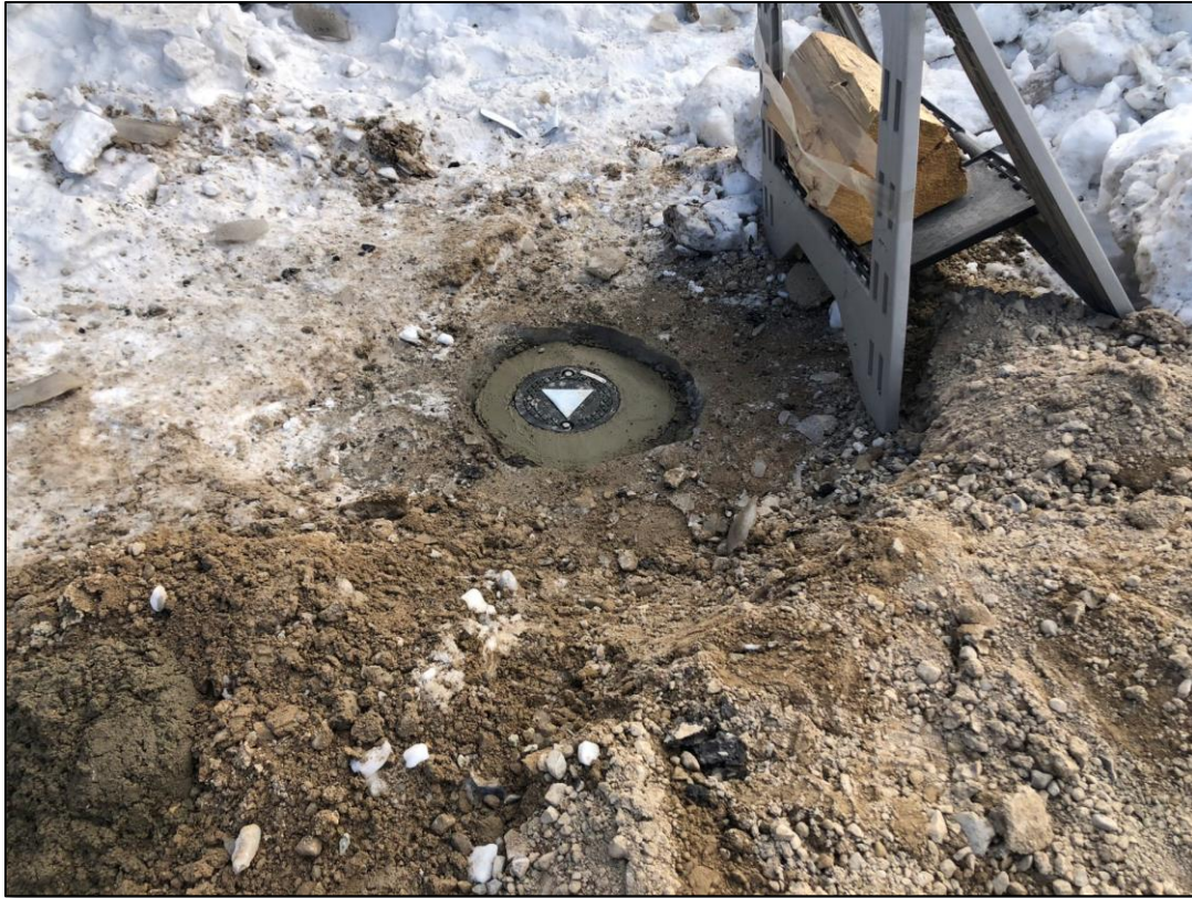
Figure 7: BH-4 Monitoring well and typical soil from borehole.
