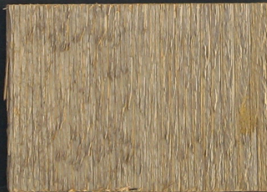
TYPICAL EXTERIOR SIDING (R.S. CEDAR W/ WEATHERING TREATMENT)
