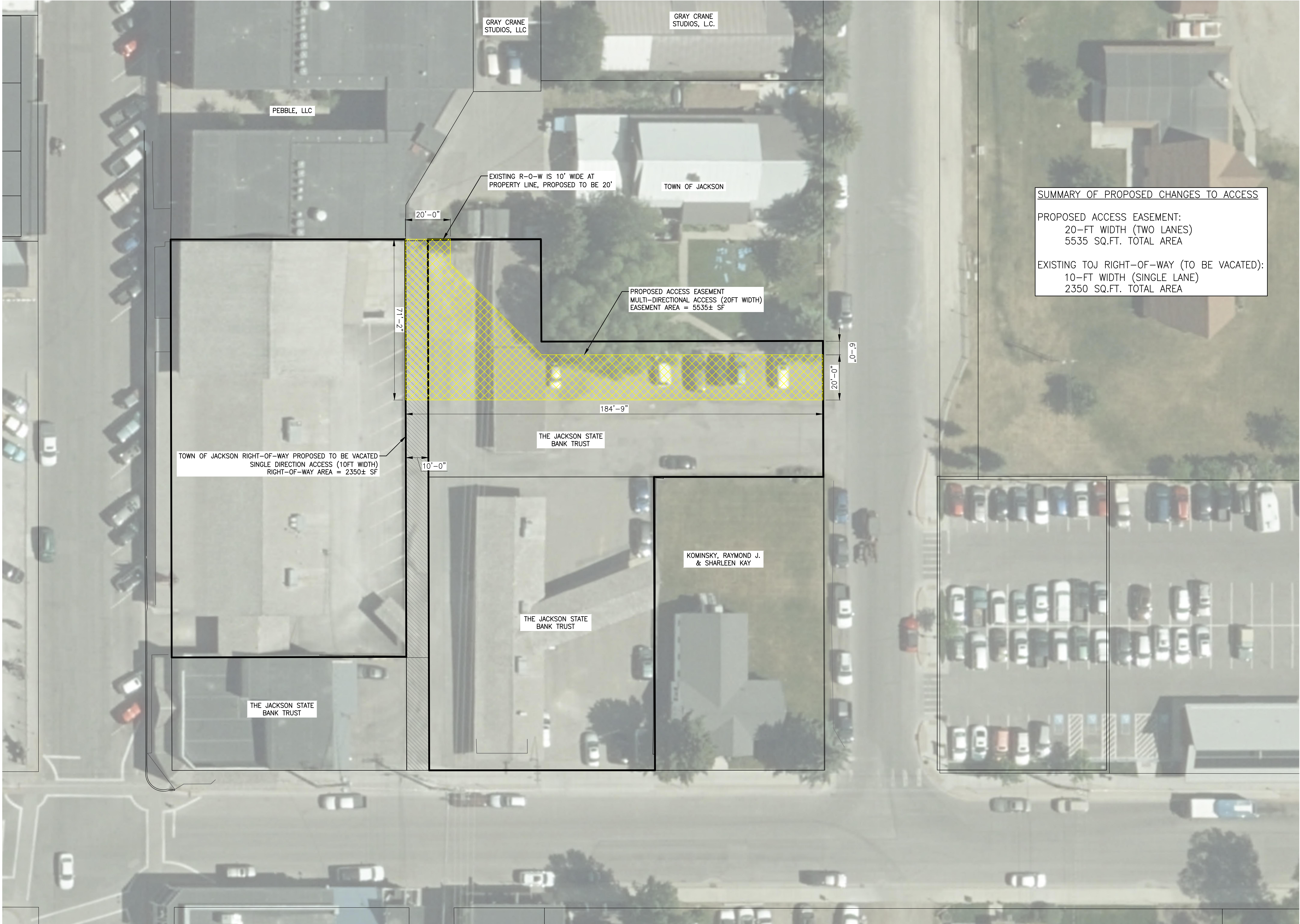
EXISTING ALLEY/PROPOSED EASEMENT EXHIBIT SCALE: 1"=20' (24x36)
